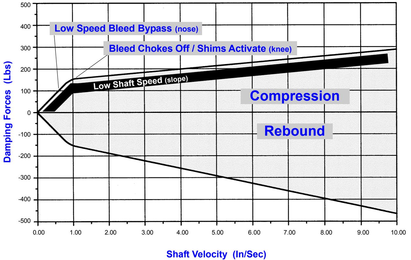
Note: Remember that low speed damping characteristics are controlled by bleed through the low speed adjuster and the bleed hole in the piston, not the valve stacks.
